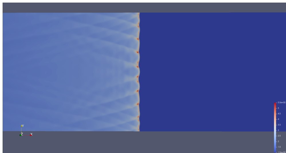
Fig. 3: Density field of two-dimensional H 2 detonation
